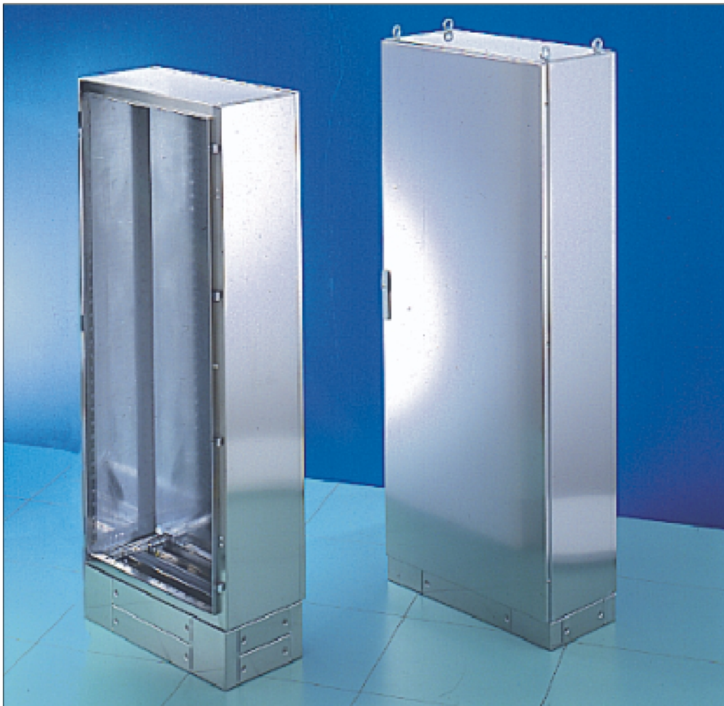
"TFR" - "TFR/V" Modular stainless steel Aisi 304, cabinets with closed sides, complete with reversible solid or transparent door/s, removable rear panel, removable bottom plates with flanges for cable entry. IP55 protection.
